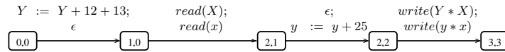
Fig. 1. A comparison transition graph for f(\&Y, y) = f^S(\&Y) \boxtimes f^T(\&y) . We use capital variables to denote the variables of the source and their lower case counterparts for the target.
