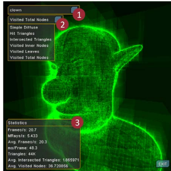
Figure 5.2: 1) A variety of scenes can be loaded through a drop-down menu. 2) 6 rendering modes are supported, with the current selection yielding a display of the number of visited nodes. 3) Statistics about scene complexity and run-time performance are supplied.
