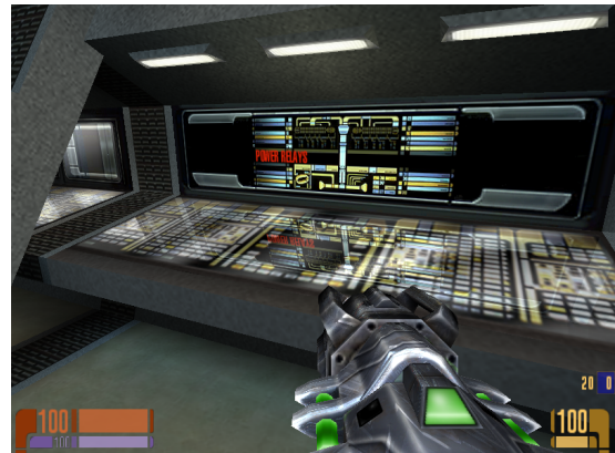
Figure 2: Raytraced reflections on a console in Raven Software's Star Trek Voyager: Elite Force, rendered at a resolution of 800x600 pixels at 2 fps on an AMD Athlon X2 3800+.
